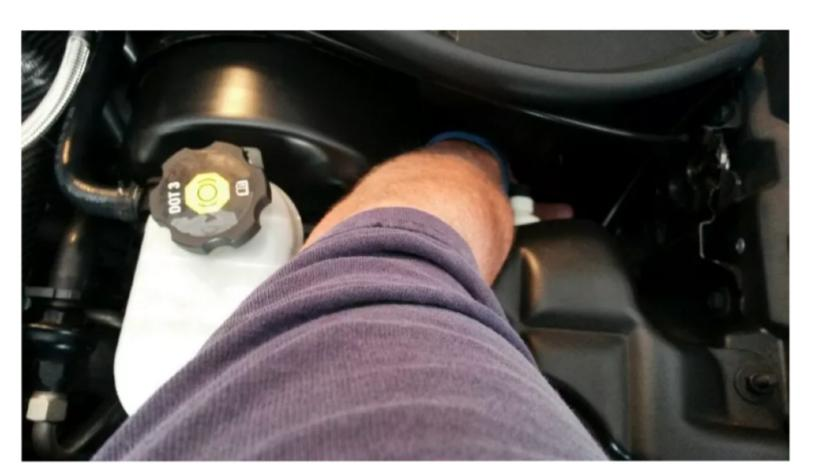
If the udders are clogged, rain and/or car wash water will not drain out of the scuttle tray. The bottom line is that the water build-up can cause a short in the electrical system in the windshield wiper motor. You may also get water on the inside of the car in the footwell area, wet rugs, or cause other problems.
